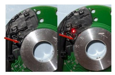
**Figure 4** The LED goes on with the S-magnet passing and off with the N-magnet passing.
