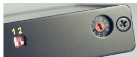
Figure 6 DIP switches and rotary switch.
