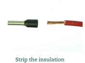
Strip the insulation off the wire end.
