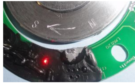
Figure 8 The LED goes on with the S-magnet passing the sensor.
