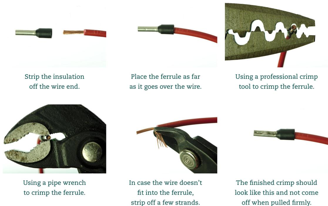
**Figure 5** Crimping the wire end ferrules.
