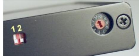
Figure 8 DIP switches and rotary switch.
