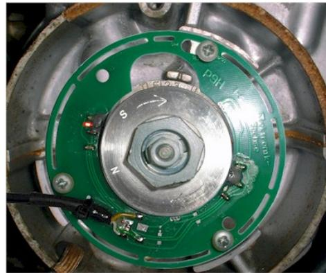
**Figure 7** The LED turns on when the S-magnet passes the sensor.
