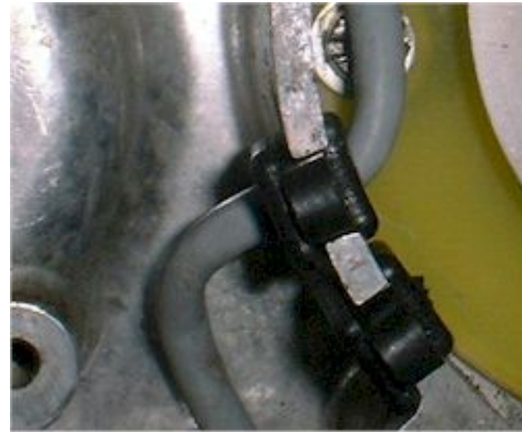
Figure 2 Route the cable through the engine case with the provided grommet.
