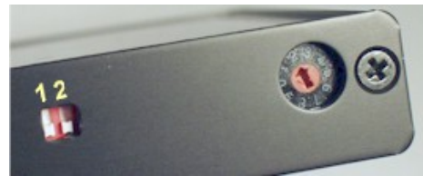
Figure 10 DIP switches and rotary switch.
