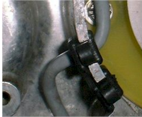
Figure 2.b Route the cable through the engine case with the provided grommet.
