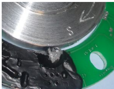
Figure 8 The LED goes off with the N-magnet passing the sensor.
