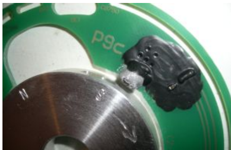
Figure 8 Position the magnet disk, so the sensor is just in front of the S-magnet.
