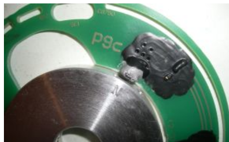
Figure 8 The LED goes off when the N-magnet passes the sensor.
