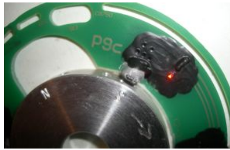
Figure 8 The LED goes on when the S-magnet passes the sensor.
