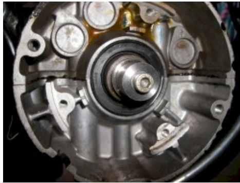
Figure 2 Assembled driver sleeve (slightly different one than the one shipped).
