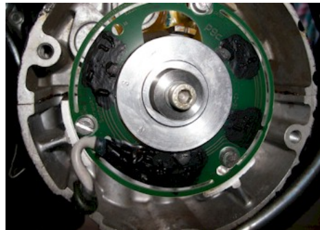
Figure 2 Installed pickup + driver sleeve + magnet disk.
