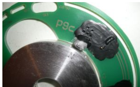
Figure 8 The LED goes off when the N-magnet passes the sensor.
