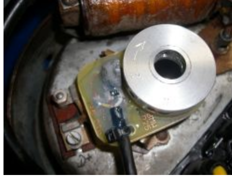
Unscrew the centre screw and tighten it again with the driver sleeve. At last push the disk onto the sleeve but don't tighten the set screws.
