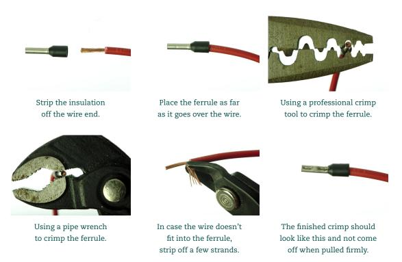
Figure 2 Crimping the wire end ferrules.
