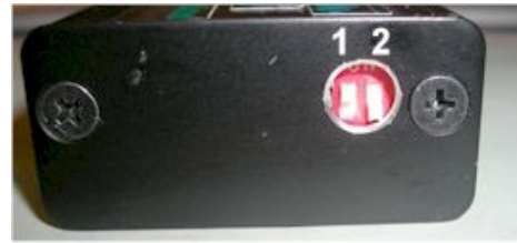
Figure 4 DIP switches and advance curve selection.
