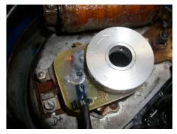
If the magnet disk happens to have two pairs of N and S magnets, it doesn't matter which pair is used for the initial setup. It is also not relevant which TDC (compression stroke or exhaust stroke) is used for the initial setup.
