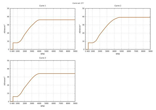
Figure 5 Selectable ignition curves.
