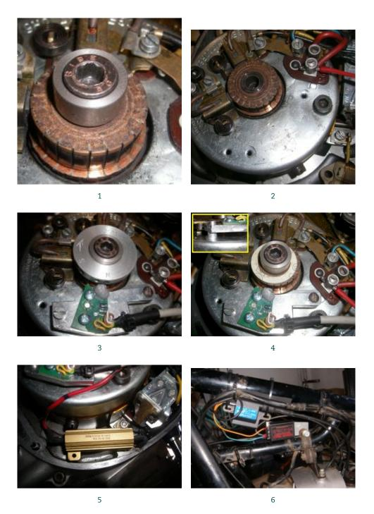
Four Brushes Alternator (12V): The mounting of the driver sleeve is identical to the above shown type. The pickup PCB is mounted with a spacing bolt on the ground terminal of a brush.
