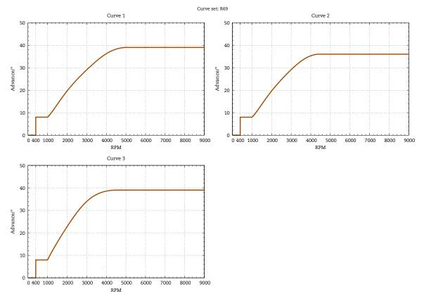
Figure 5 Selectable ignition curves.
