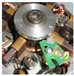
If the magnet disk happens to have two pairs of N and S magnets, it doesn't matter which pair is used for the initial setup. It is also not relevant which TDC (compression stroke or exhaust stroke) is used for the initial setup.
