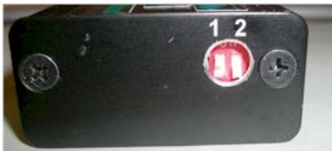
**Figure 4** DIP switches and advance curve selection.
