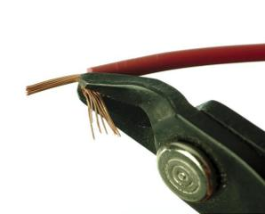
In case the wire doesn't fit into the ferrule, strip off a few strands.
