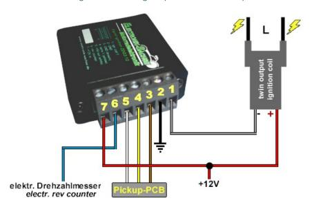
Table 2 on page 8 details how the ignition box is wired up.
