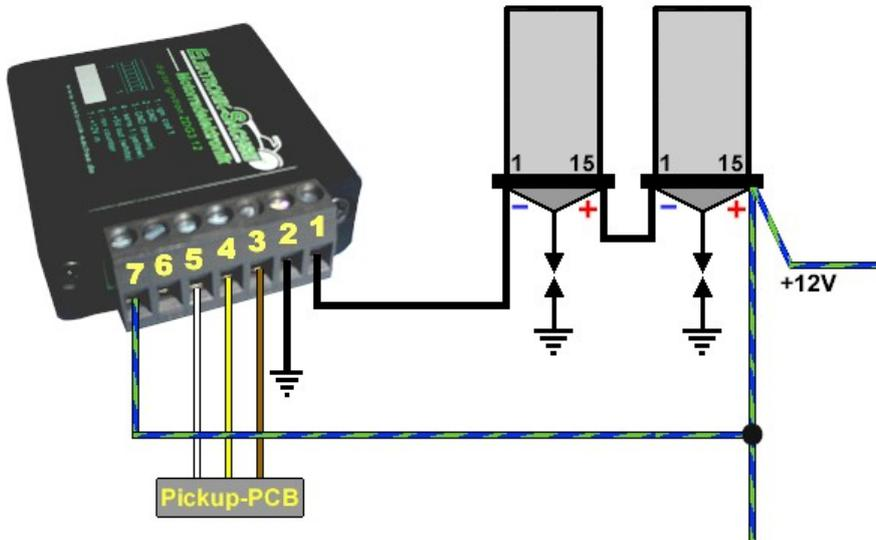
Ignition circuit diagram (two 6V coils in series)
