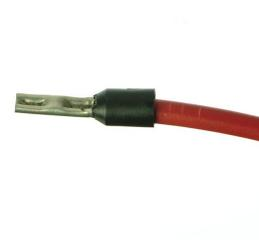
The finished crimp should look like this and not come off when pulled firmly.
