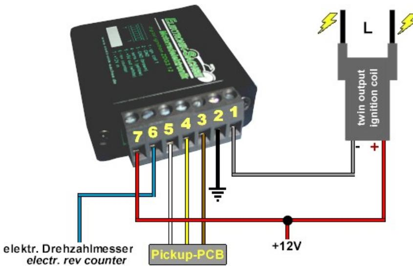
Table 2 on page 8 details how the ignition box is wired up.
