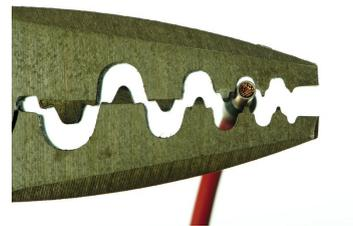
Using a professional crimp tool to crimp the ferrule.
