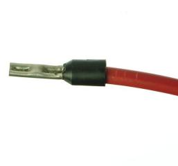
The finished crimp should look like this and not come off when pulled firmly.
