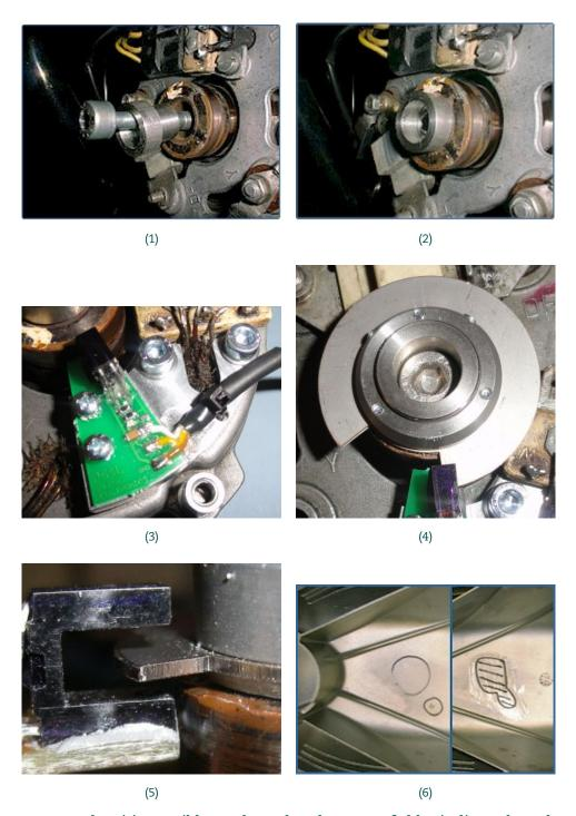
Note that it's possible to short the alternator field winding when the sector disk is touching the rotor. Therefore ensure that the sector disk maintains some clearance to the rotor.
