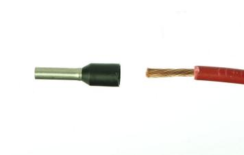
Strip the insulation off the wire end.
