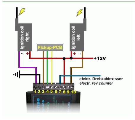
Ignition circuit diagram with two 12 V coils.
