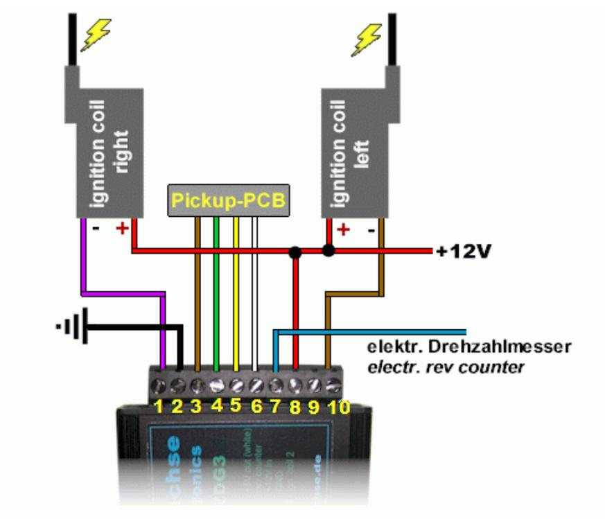
Ignition circuit diagram with two 12 V coils.
