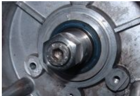
Figure 2.d The driver sleeve is held in place with the centre bolt.
