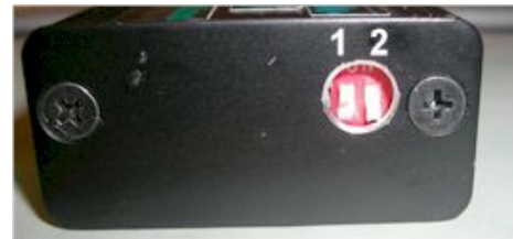
Figure 5 DIP switches and advance curve selection.
