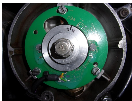
Figure 2.e Mounting the new pickup, driver sleeve and magnet disk. The set screws in the magnet disk need not be tightened at this point, yet.
