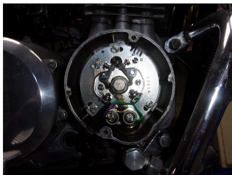
Figure 2.a The old components of the ignition can be removed as they are no longer required and replaced by the parts in the kit.
